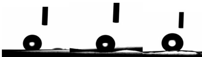
Figure 10. Contact angle of water on preparations of 5 electrospun from DMF (left, 140°), 5 electrospun from chloroform (middle, 121°), and 6 electrospun from chloroform (right, 149°).
